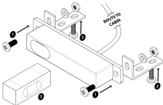
1. Using bolts, nuts and washers, mount the sensors to supplied L-shaped brackets, and tighten them firmly.
